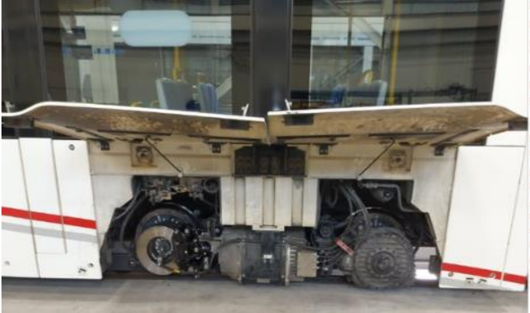
Bogie installed on a LRV
