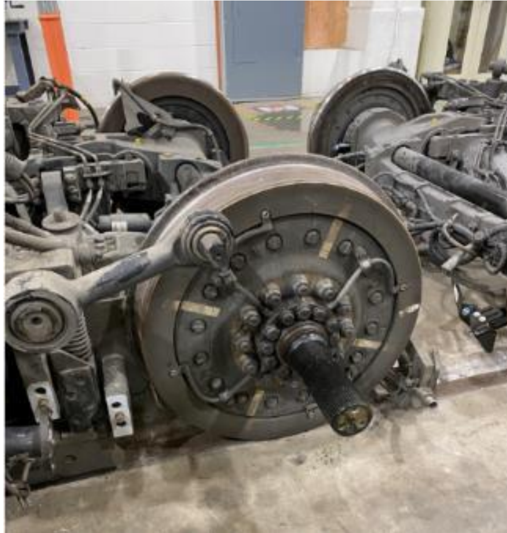
Bogie with gearbox removed (undamaged)
