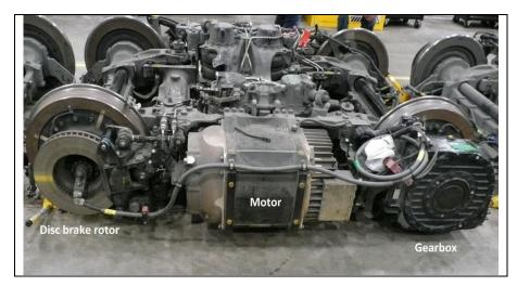
Each motor bogie is equipped with 2 motors—1 on each side of the bogie. Power from each motor is transmitted to a drive wheel through a gearbox that interconnects with a splined axle stub, also referred to as a reducer hub, which is secured to the wheel hub with 12 bolts (Figure 3). Disc brake rotors are attached to the wheel hub opposite the drive wheel of each motor bogie wheel set (Figure 4), and to each wheel of the trailer bogies. The rotors are also secured to the wheel hub with 12 bolts.
