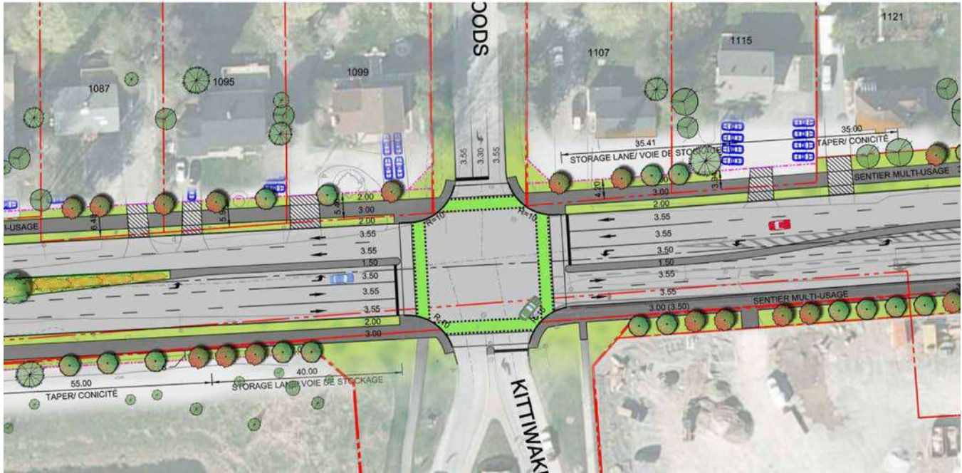
Figure 6-3: Alternative A - Signalized Intersections, Kittiwake Drive/Echowoods Avenue
